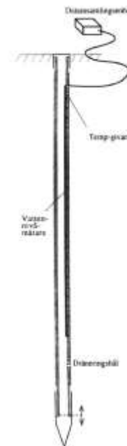
Figure 5.1. VTI team installing the STÖR-96 instrument on January 8, 1997 in Sweden (left) and its principal scheme (right).
