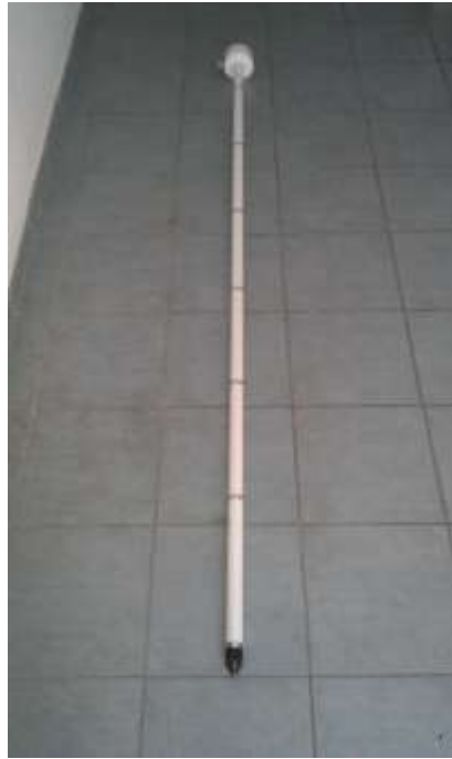
Figure 5.4. Lithuanian RWSs temperature probe PT100 with a highly stable and accurate platinum sensing element.
