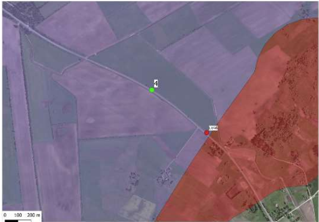
Figure 5.21. Monitoring station 4. Legend: Green dot – monitoring station; Red dot – weather monitoring station; brownish red colour represents glacial sediments, purple colour represents glaciolimnic sediments (Ortho photo mosaic base map).
