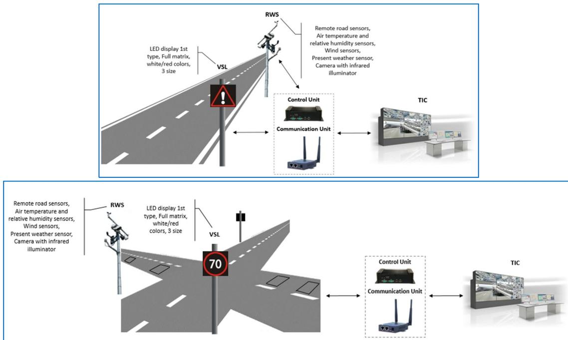
**Fig. 3.** Examples of VMS system subtypes, approved for LSR: VMS/RWS combined installation (above) and traffic calming VMS for crossing at grade (below)
